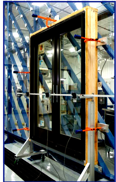
Test sample prepared for structural testing using precision digital deflection transducers
